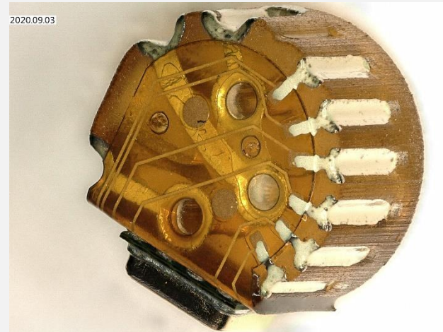
Catheter tip with a diameter of 4.5mm, combining 3D plastic printing, aerosol jet printing, thinfilm circuit manufacturing and microsystem assembly
