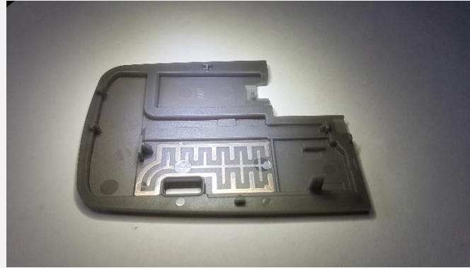
Capacitive sensor for on body detection of (medical) devices
