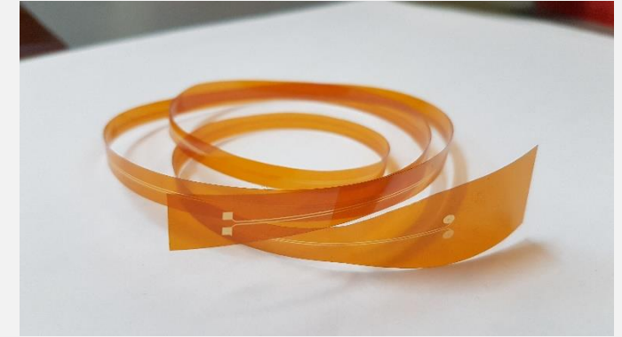
Bio-compatible gold structures printed on plastic foils, used for neurostimulation
